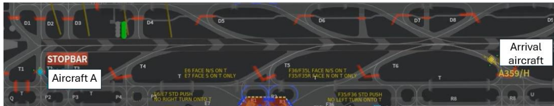
Figure 2: STOPBAR visual alert on ASMGCS.
